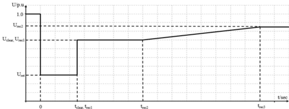
**Figure 6C.** Fault-ride-through profile of a type C synchronous power-generating module
