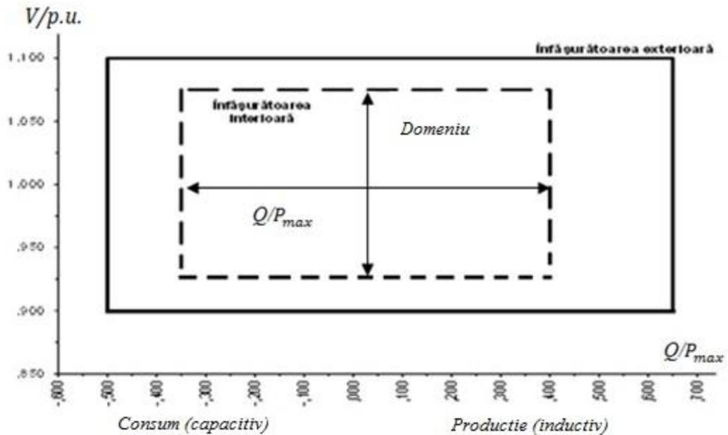
**Figure 7C.** U- $Q/P_{max}$ -profile of a synchronous power-generating module
