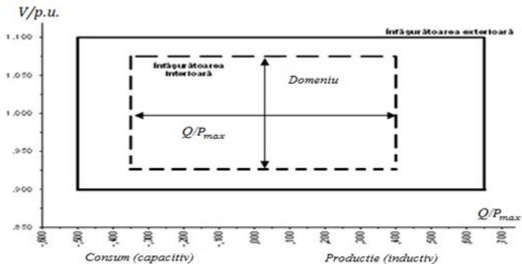
**Figure 7D.** U- $Q/P_{max}$ -profile of a synchronous power-generating module
