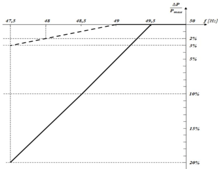
**Figure 2C.** Admissible limits for power reduction established by the TSO in case of underfrequency
