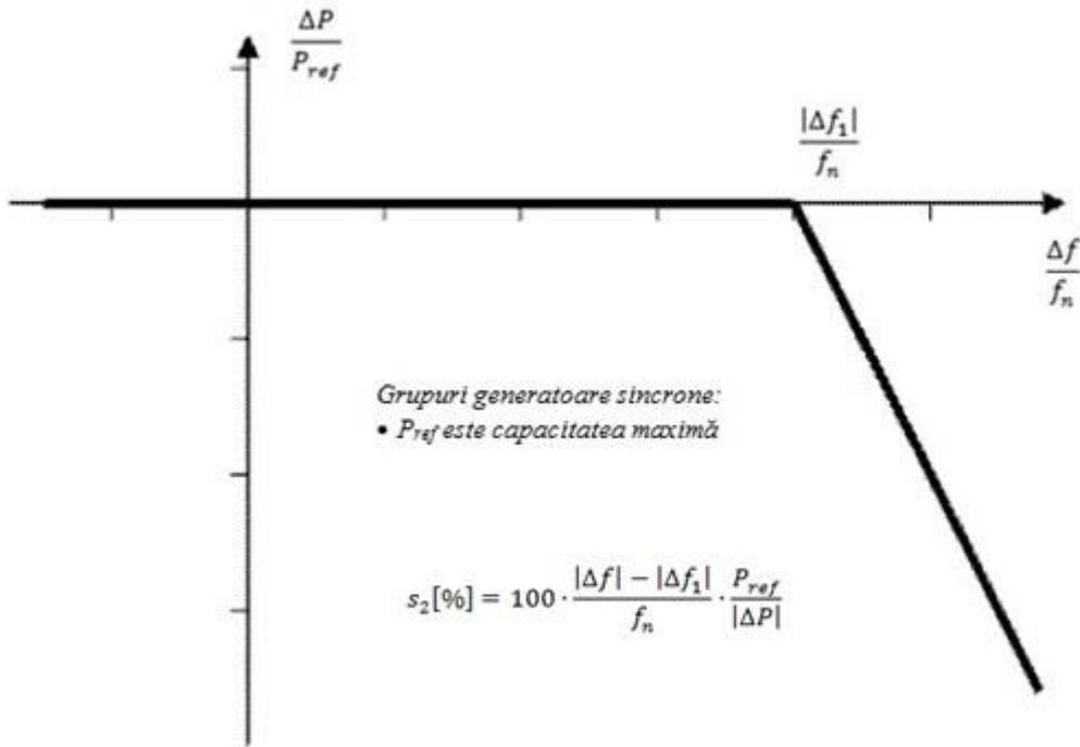
**Figure 1C.** Active power frequency response capability of type C synchronous power-generating modules in LFSM-O
