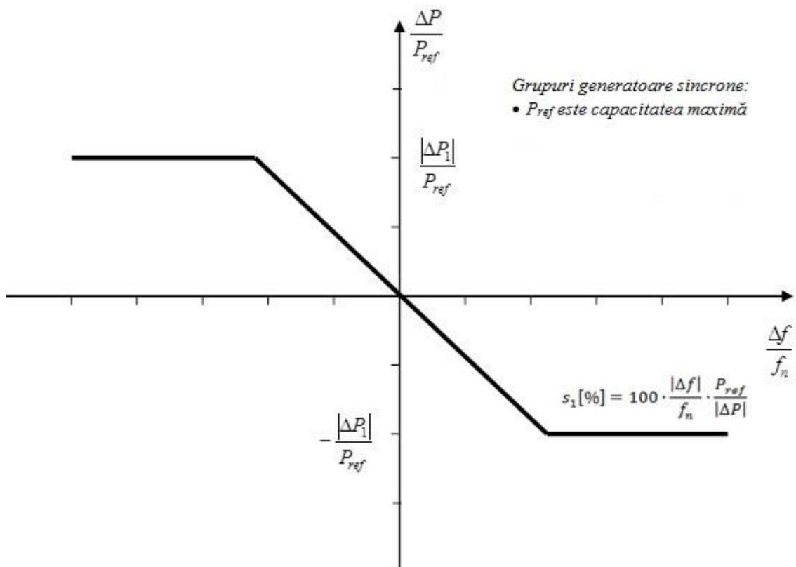
**Figure 4C.** Active power frequency response capability of type C synchronous power-generating modules in FSM illustrating the case of zero deadband and insensitivity area.
