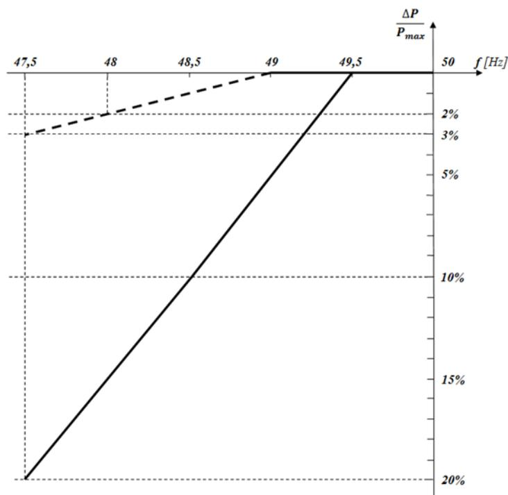
**Figure 2A.** Admissible limits for power reduction established by the TSO in case of underfrequency
