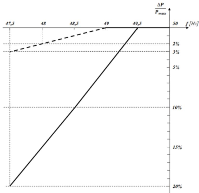
**Figure 2B.** Admissible limits for power reduction established by the TSO in case of underfrequency
