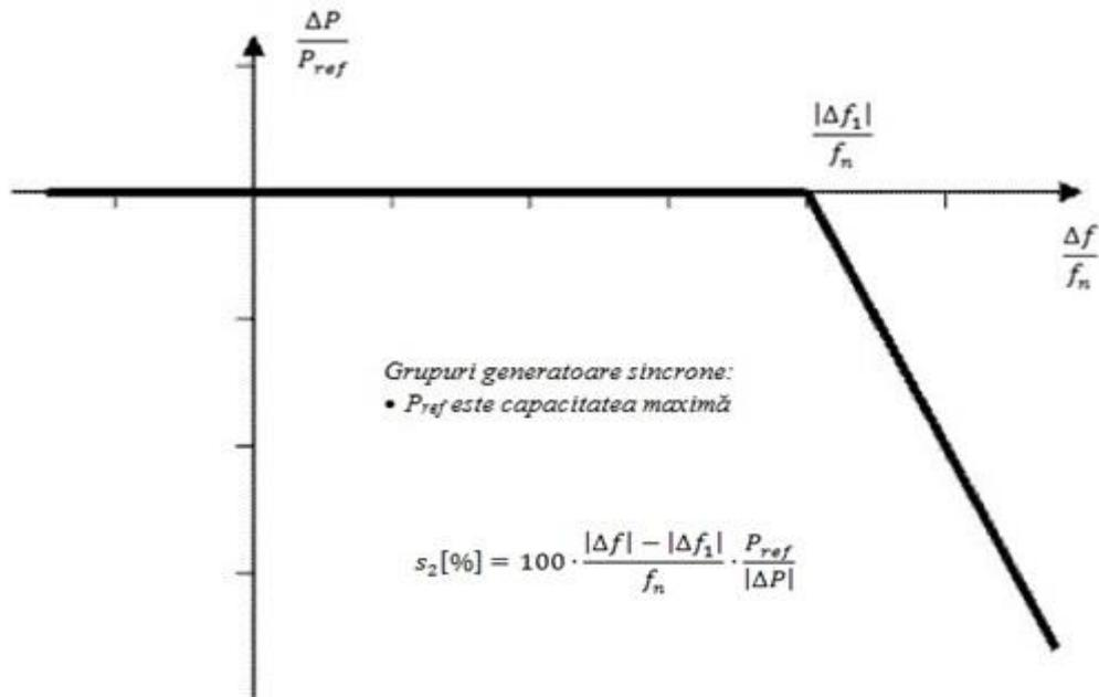
**Figure 1D.** Active power frequency response capability of type D synchronous power-generating modules in LFSM-O
