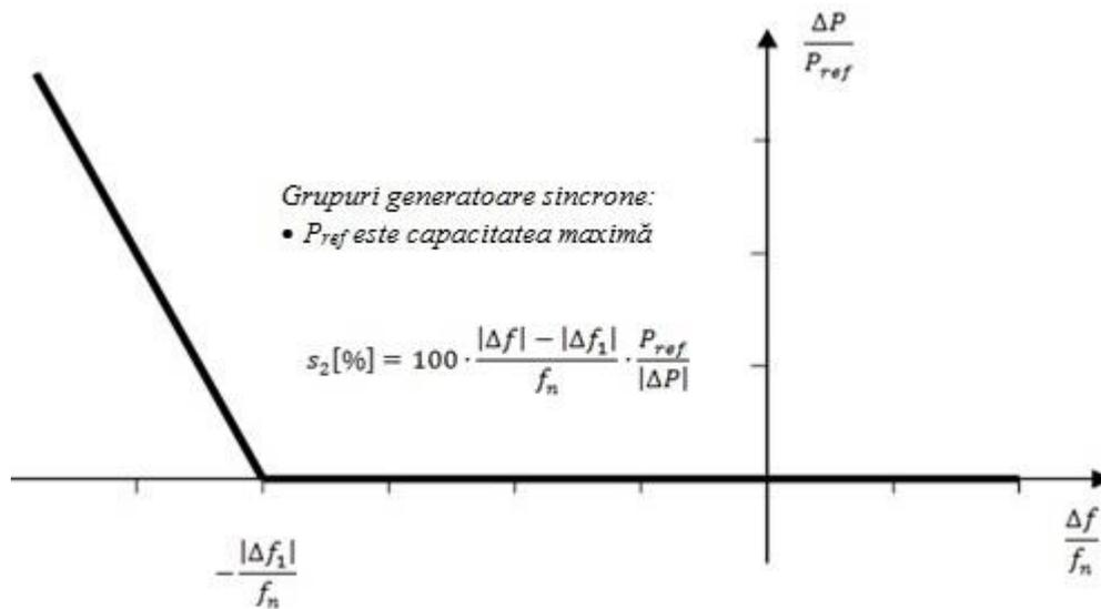
**Figure 3C.** Active power frequency response capability of type C synchronous power-generating modules in LFSM-U
