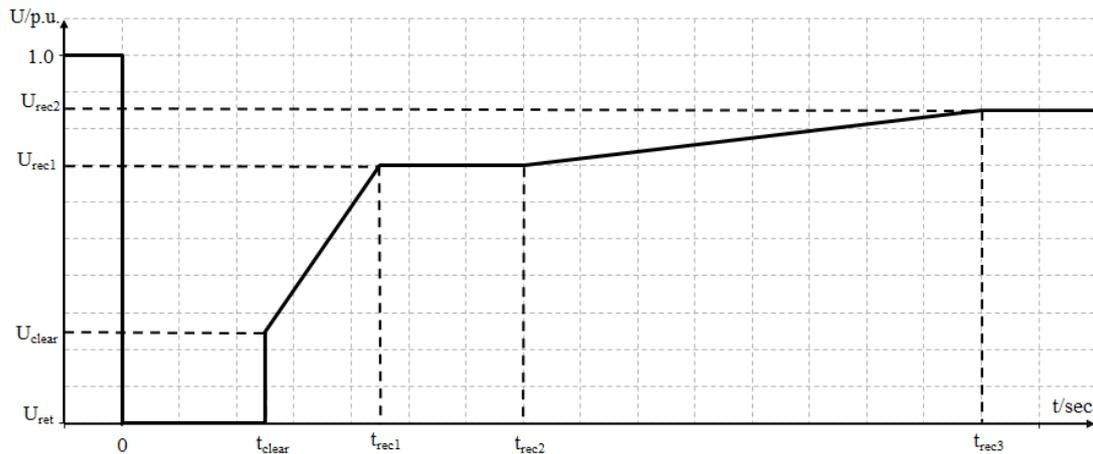
**Figure 6D.** Fault-ride-through profile of a type D synchronous power-generating module
