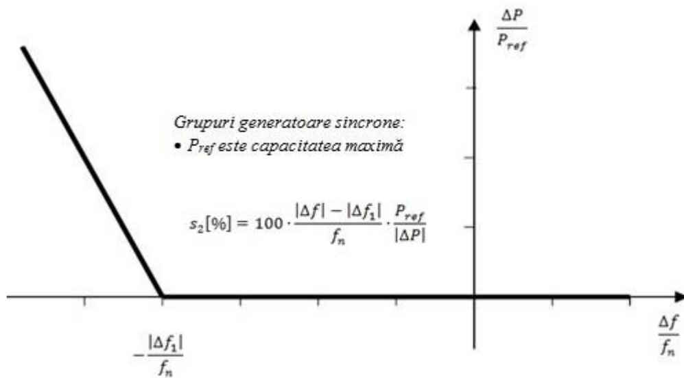
**Figure 3D.** Active power frequency response capability of type D synchronous power-generating modules in LFSM-U
