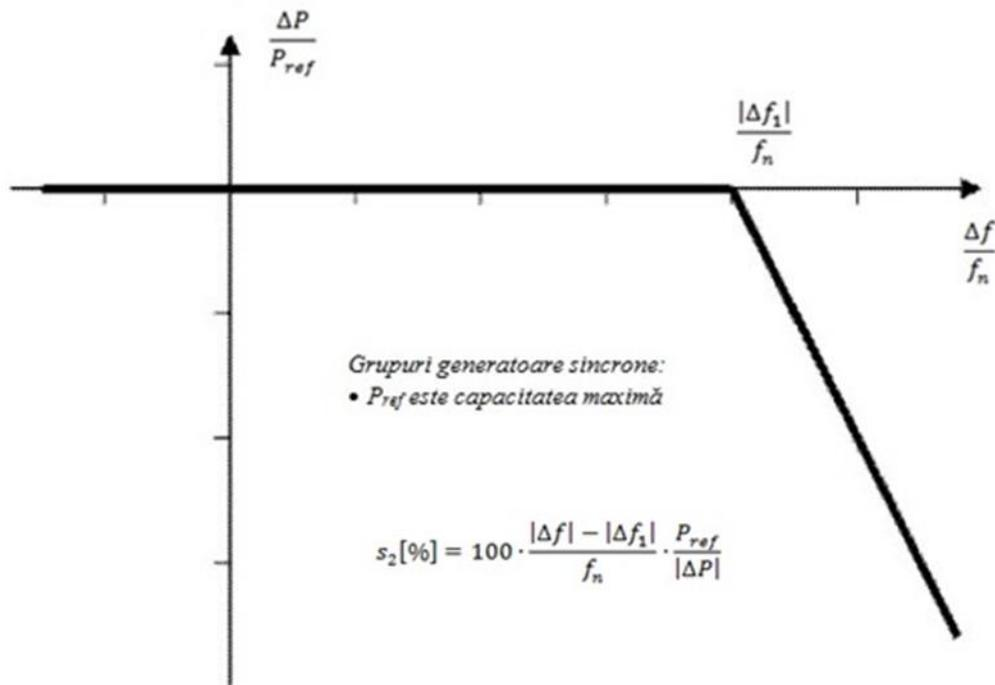
**Figure 1A.** Active power frequency response capability of type A synchronous power-generating modules in LFSM-O
