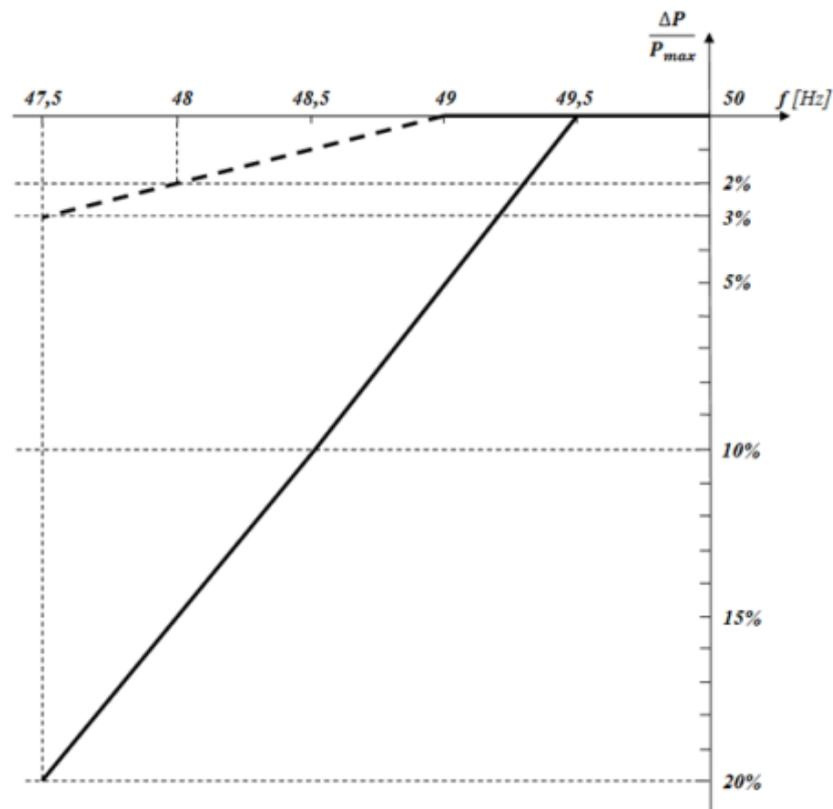
**Figure 2D.** Admissible limits for power reduction established by the TSO in case of underfrequency
