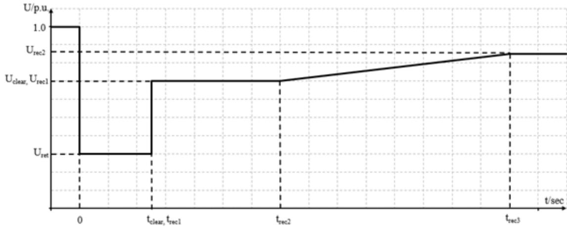
**Figure 3B.** Fault-ride-through profile of a type B synchronous power-generating module
