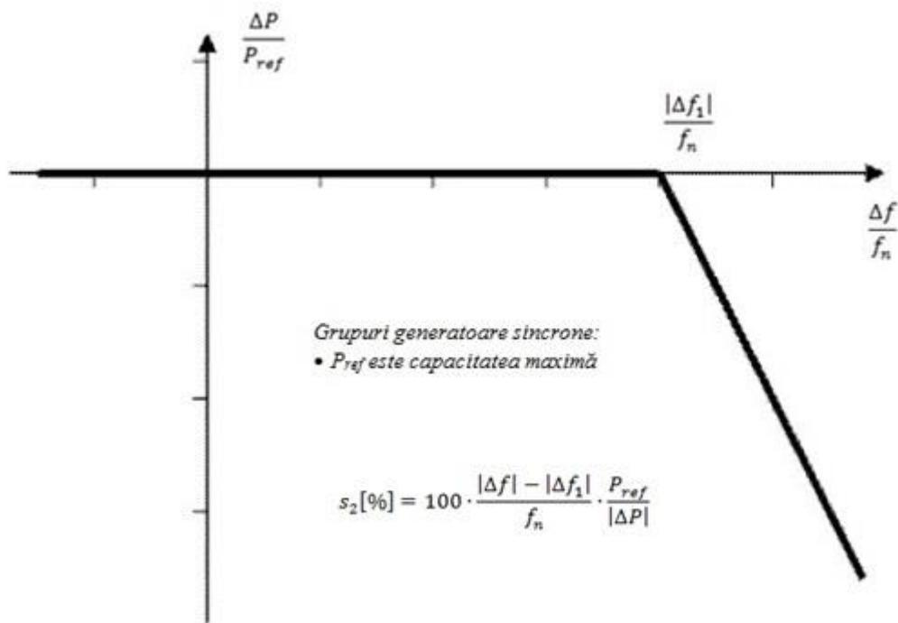
**Figure 1B.** Active power frequency response capability of type B synchronous power-generating modules in the LFSM-O mode
