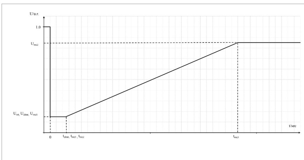
**Figure 3B.** Fault-ride-through profile of a type B power park module
