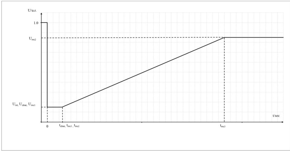
**Figure 6C.** Fault-ride-through profile of a type C power-generating module
